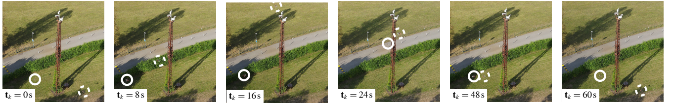
Figure 9: Snapshots of the power tower inspection scenario. The system evolution at different time instants t_k is reported. Solid and dashed circles are used to indicate “drone1” and “drone2”, respectively.
